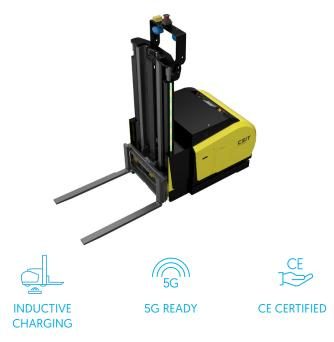
An autonomous forklift AMR with counterbalance and a lifting height of up to 6 metres. Its high degree of modularity and scalability makes it suitable for use in various production or warehouse premises.
